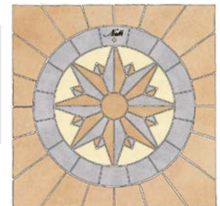
When laying circles always lay from the centre outwards. We advise first laying out dry to determine optimum spacings before fixing on mortar.
