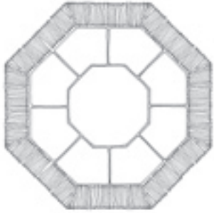
ME18 Width 1.92m Components: 1 no. Octant Centre Stone 8 no. Petite Octant Cornerstone 8 no. Octant Corner Tile on Edge 8 no. Straight Tile on Edge
